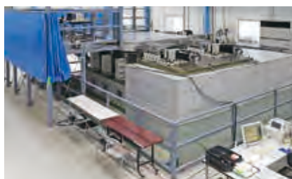
Large-Scale Triaxial Vibration Test System Railway vehicle standards, earthquake simulation compatible Table size: 2800 × 2800 mm
