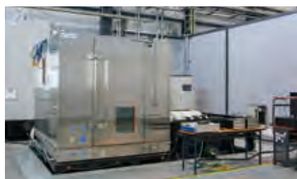
200 kN Large-Scale Vibration-Temperature Combined Environmental Reliability Test System Maximum excitation force: 200 kN Table size: 2000 × 2000 mm
