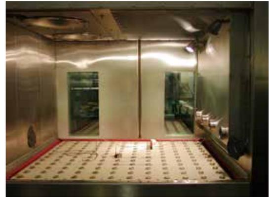
HALT/HASS testing challenges the design, components, sub-assemblies and final assemblies of today's manufactured products. Stresses are applied through a number of conditions to set operational limits and ultimately precipitate failure in the HALT/HASS test environment. Rapid thermal change rate is one of the classic conditions that facilitate product stress.
