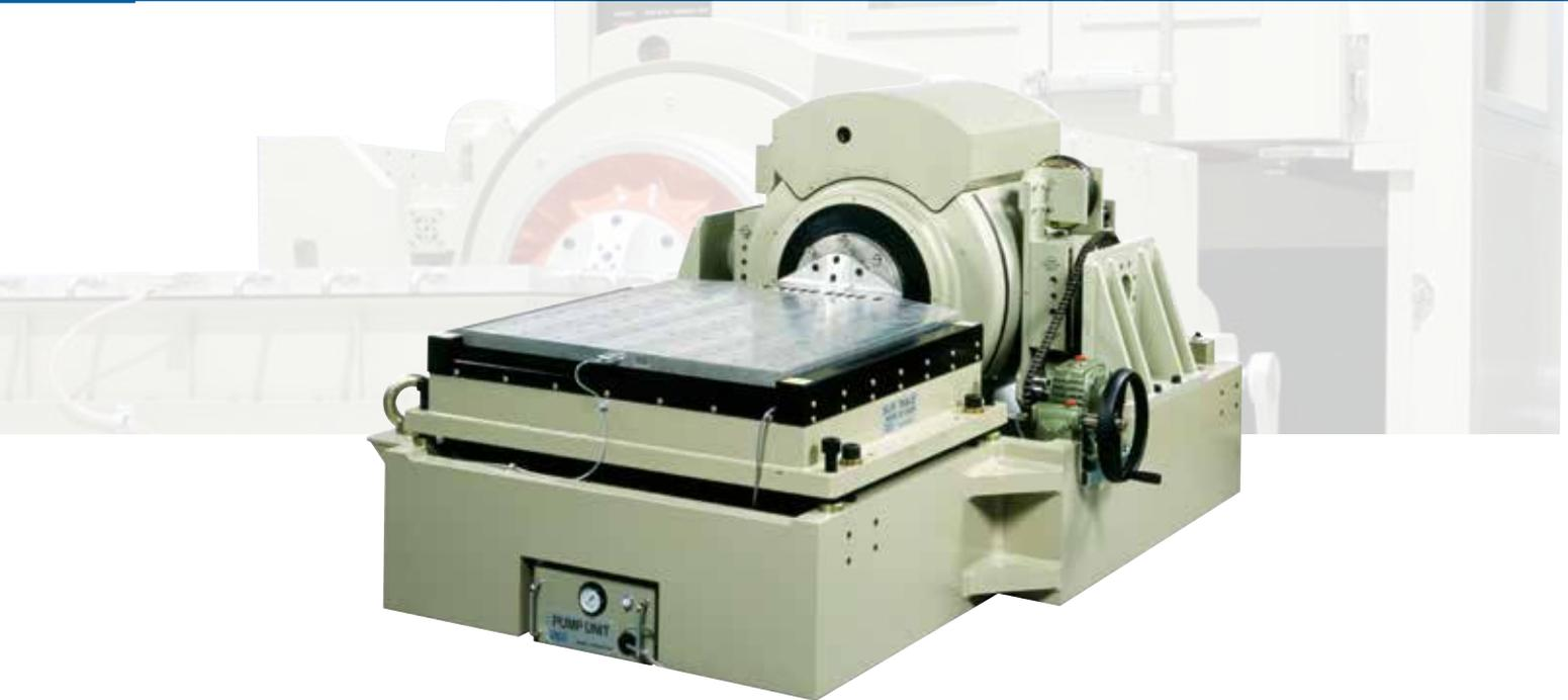
The slip table system is the most familiar option to perform horizontal testing of a bulky unit or an article, which the mounted configuration cannot be changed. It has many uses for various tests such as: transportation test of electrical appliances, computers and office equipment, durability test of railway rolling stocks, signaling equipment and automobile parts, and environmental test of aeronautical equipment.
