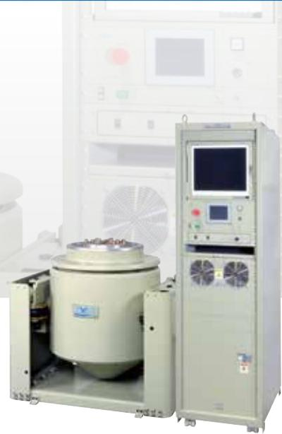
The FL series system expands the maximum displacement to 100 mm<sub>p-p</sub>. In particular, it responds to the test condition of large displacement of less than 10 Hz.
